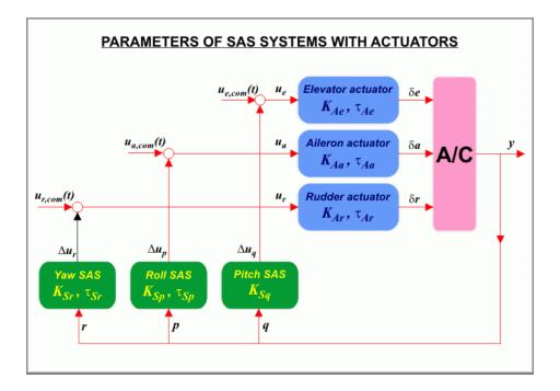
Figure 32: Closed loop feedback system
