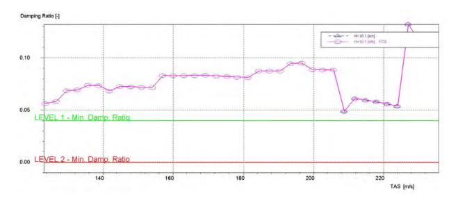
Figure 33: Phugoid mode damping ratio with respect to TAS (MIL standard)
