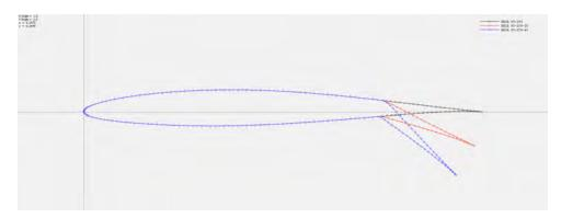
Figure 16: NACA 63209 with different flaps settings
