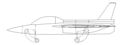
Figure 21: Undercarriage retraction
