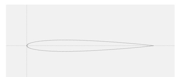
Figure 15: NACA 0009 airfoil
