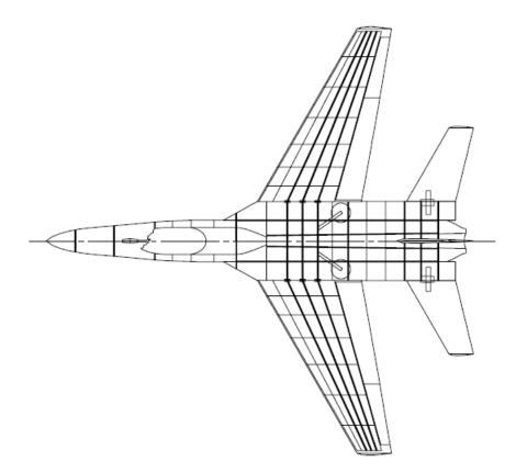
Figure 59: Top view of aircraft and structure elements
