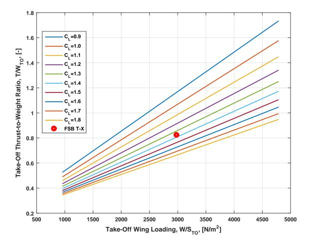
Figure 9: Lift coefficient with take-off requirements, A=5
