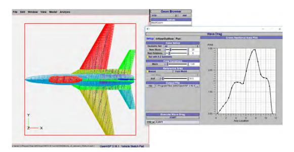
Figure 40: Wave Drag shown in OpenVSP
