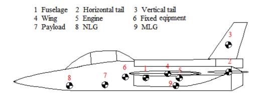
Figure 25: Side view of CG positions
