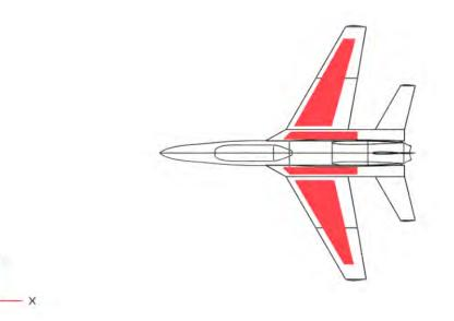
Figure 55: Fuel tank storage in the aircraft
