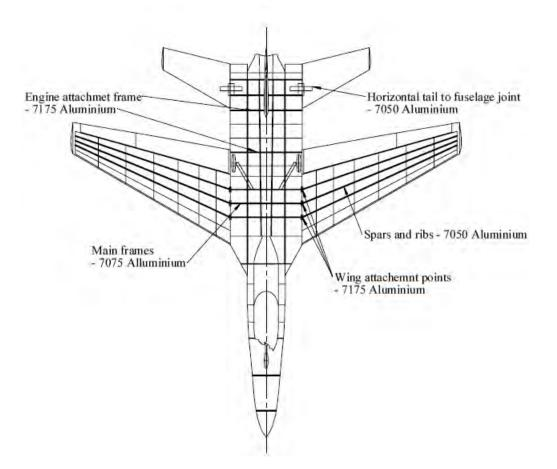
Figure 61: Aircraft parts and materials in the ground plan
