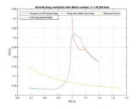
Figure 41: Drag coefficient with Mach number
