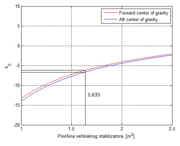
Figure 29: Rudder feedback gain
