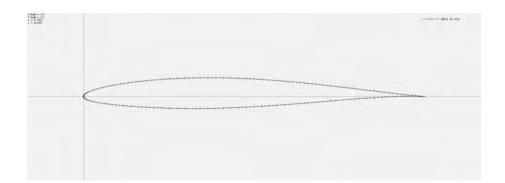
Figure 13: NACA 63209 with 200 panels
