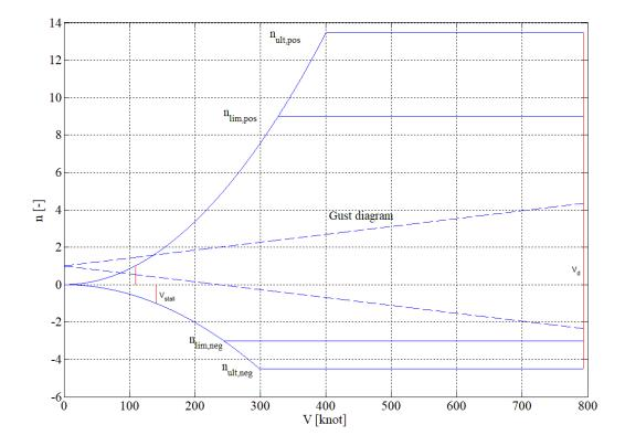
Figure 58: V-n diagram
