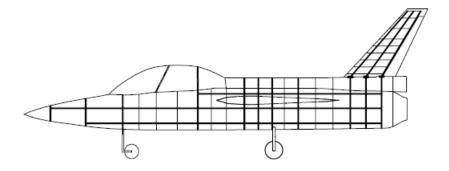
Figure 60: Side view of aircraft and structure elements
