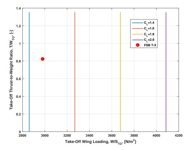
Figure 10: Lift coefficient with landing requirements, A=5
