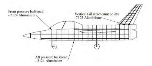
Figure 62: Parts and materials of the aircraft in the side view
