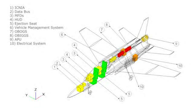
Figure 56: Layout of basic aircraft systems
