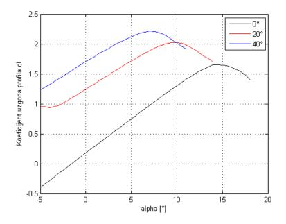
Figure 17: Section lift increase for different flaps settings
