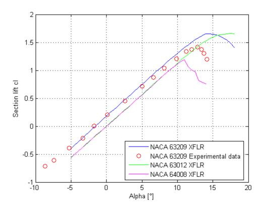
Figure 14: Comparison of section lift for different NACA 6-series airfoils
