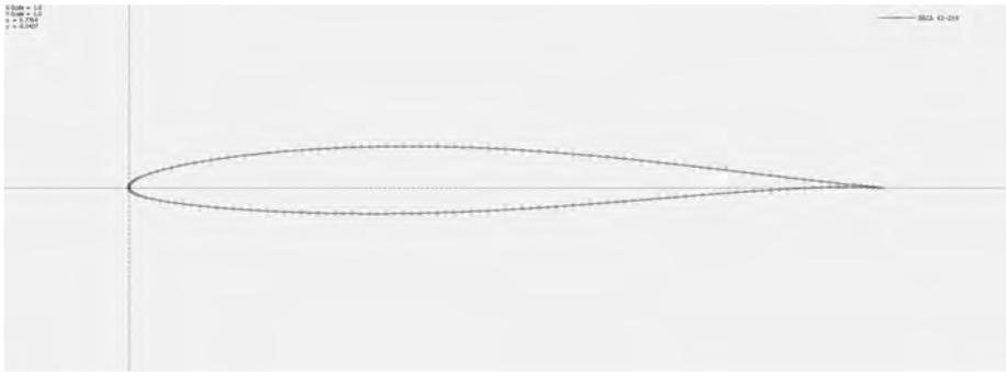
Figure 13: NACA 63209 with 200 panels
