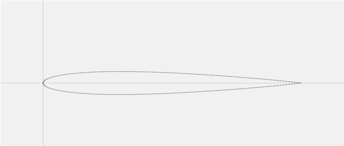
Figure 15: NACA 0009 airfoil
